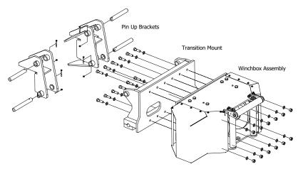
NOTE: Recovery winch only. Not to be used for towing. U.S. Patent No. 11,926,990
