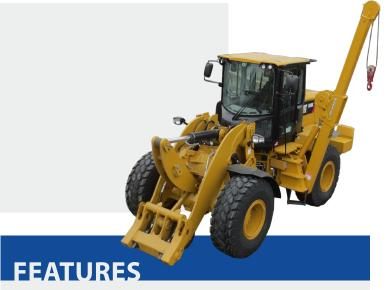
Three lever cable control allows simultaneous, precise control of the load and boom functions. The controls are easy to operate and require minimal operator training.
