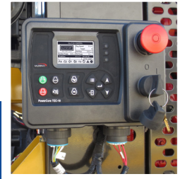
Operator's Control Station
